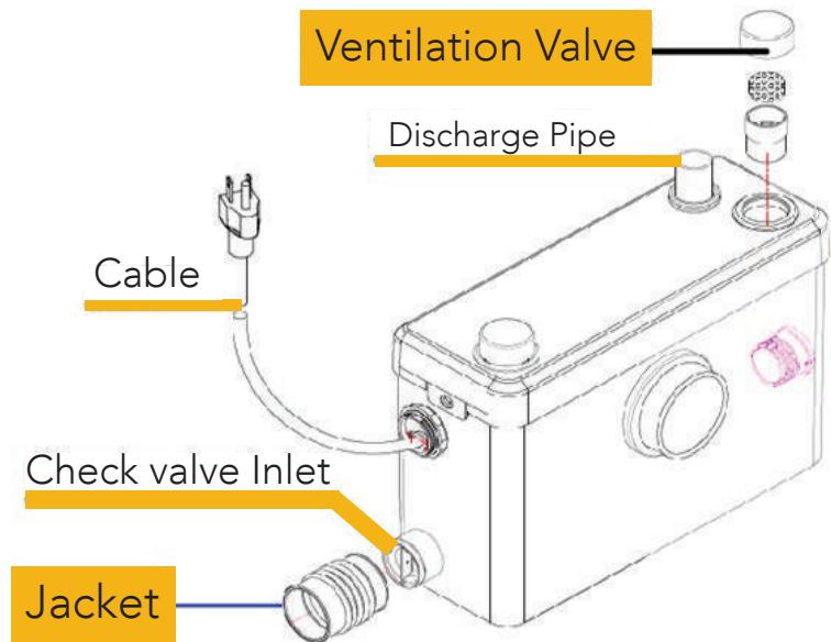
The drawing example is for the normal layout as the bathroom application : Toilet, Bathtub and Sink
